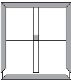
INSTALL CORNER SUPPORTS AT BOTH ENDS OF THE BOTTOM PERIMETER AND WORK THE CORNER SUPPORTS IN A LITTLE AT A TIME FROM BOTH SIDE UNTIL THE PERIMETER CAN BE INSERTED INTO THE BRACE
