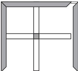
INSTALL CORNER SUPPORT AND JOIN THE TOP PERIMETER AND BRACE
